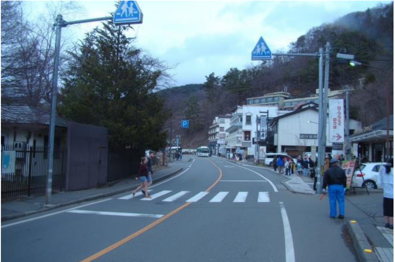
Figure 6.63 - Stop lines 5 to 10 m before an unsignalized crosswalk in Kawaguchiko, Japan.
