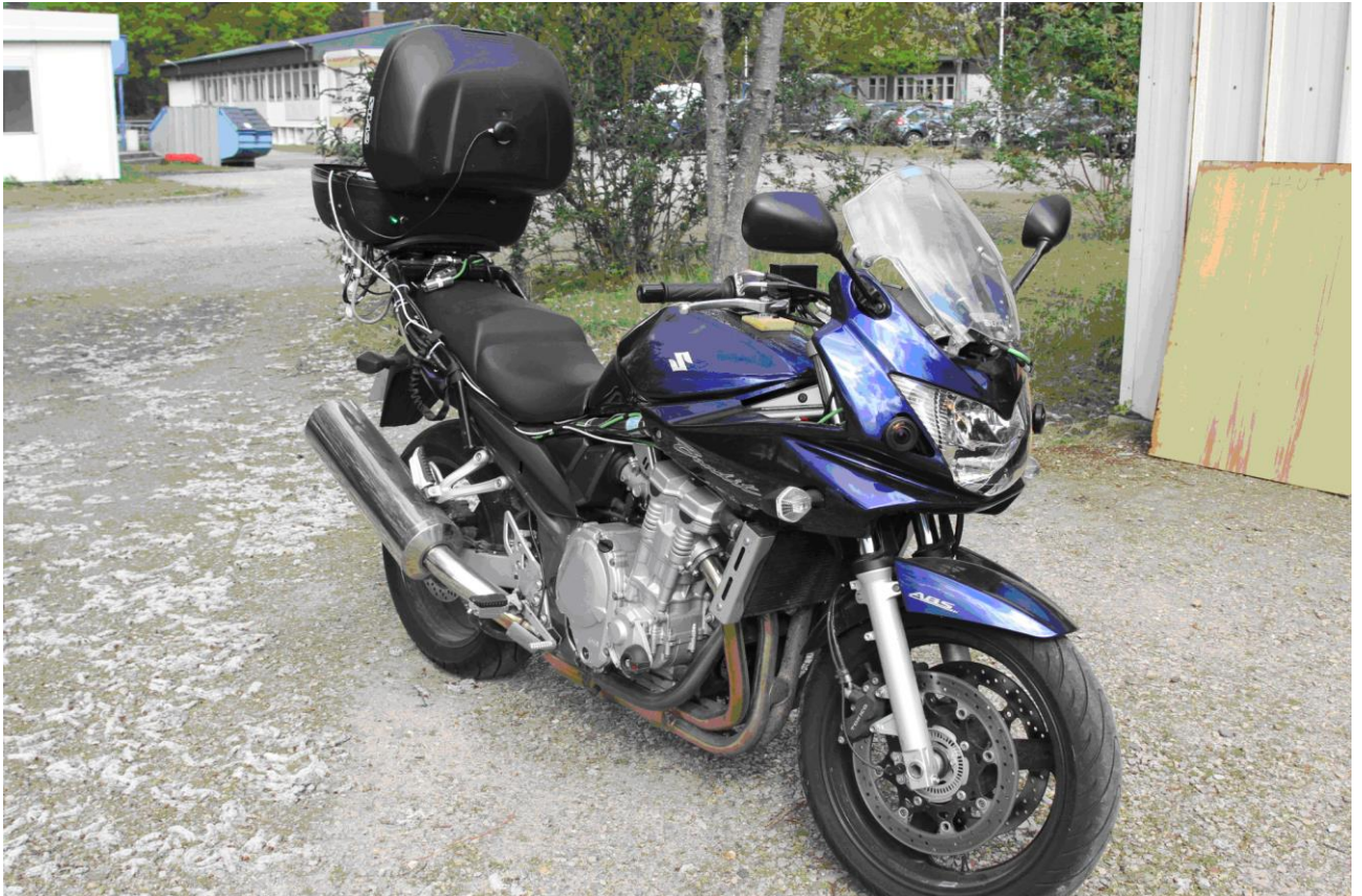
Figure 6.136 - The instrumented motorcycle (called MACC)
