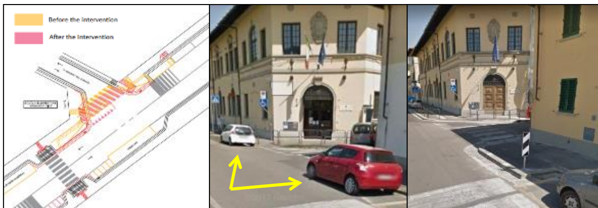
Figure 6.85 - Site 2, situation before the intervention (in the centre) highlighting two cars parked immediately before the two zebra crossing, and situation after the intervention (on the right) [1] [2]
