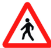
Figure 6.141 - P-20 Road Sign: Danger due to the proximity of a place frequented by pedestrians
