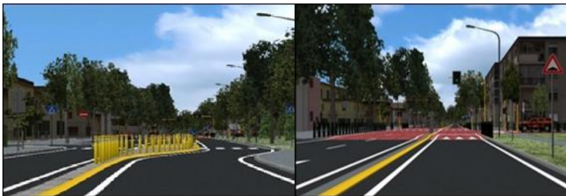
Figure 6.159 - Details of the designed countermeasures: on the left, yellow bollards in a change of the cross section, on the right, a raised coloured intersection. Both the countermeasures capture drivers attention alerting them of a critical point and moving the focal point closer.
