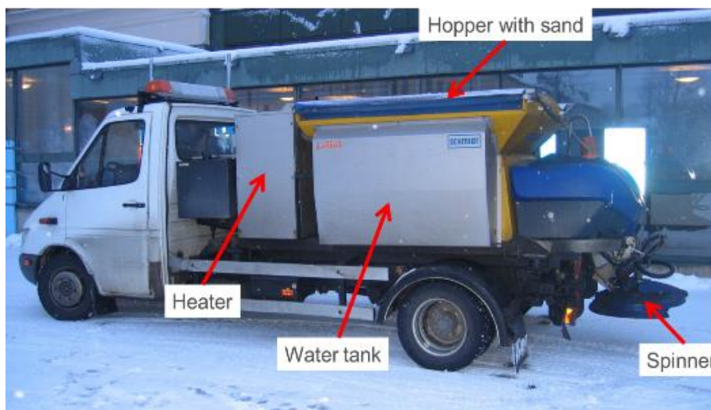
Figure 6.153 - The equipment used for spreading warm wetted sand on walkways and bike paths in Umeå municipality, in Sweden.
