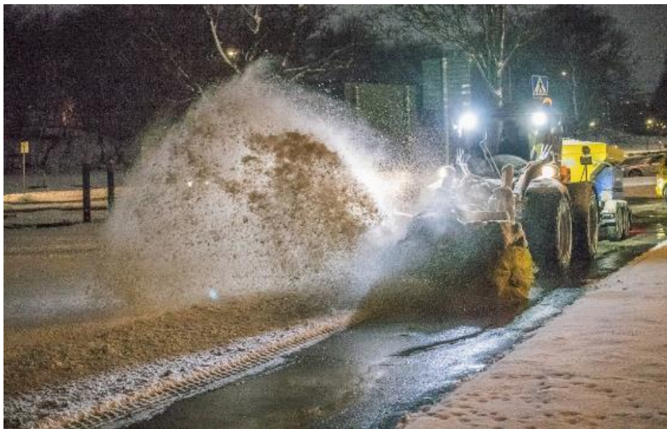
Figure 6.152 - A sweep sweep-salting measure on a bicycle path in Stockholm
