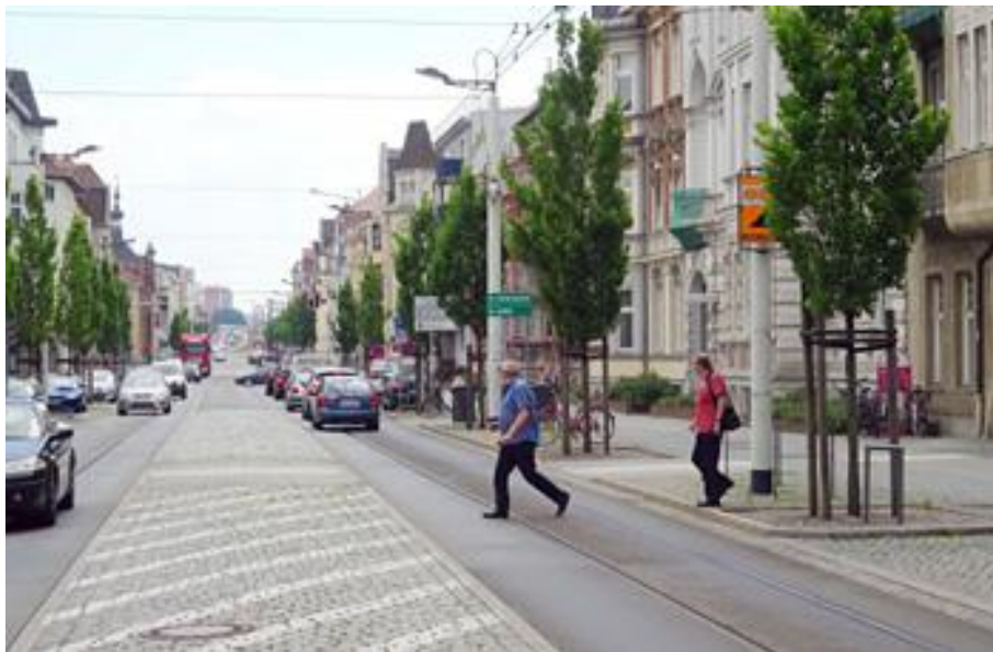
Figure 6.24 - The medial strip as a crossing aid for pedestrians, source: Stadt Cottbus
