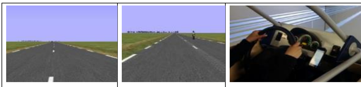
Figure 6.212 - Views of the three driving situations. At left, the reference situation without traffic. At centre, the overtaking of two powered wheels. At right, SMS writing: word “juin” (copyright Ifsttar, 2012)
