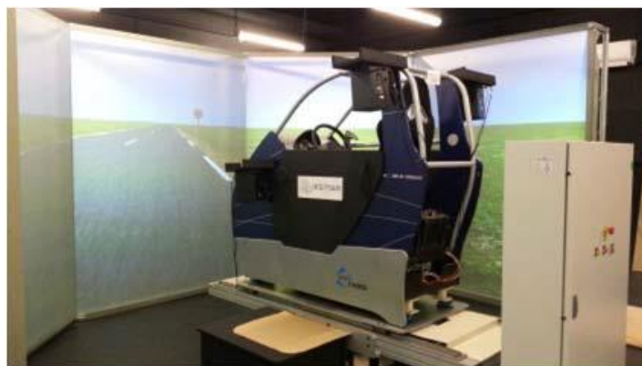
Figure 6.211 - View of the fixed-base driving simulator (copyright Ifsttar, 2012)
