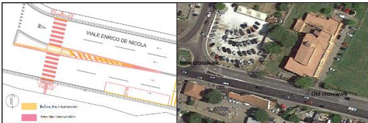
Figure 6.69 - Intervention on site 2, moving of the crosswalk position close to the roundabout intersection [4] [5]
