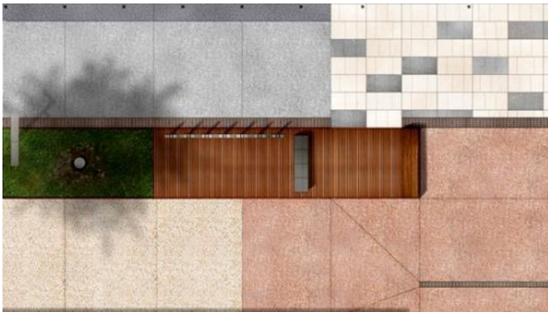
Figure 6.222 – Detail of the junction between the cycle path and raised pedestrian crossing (square) [5]
