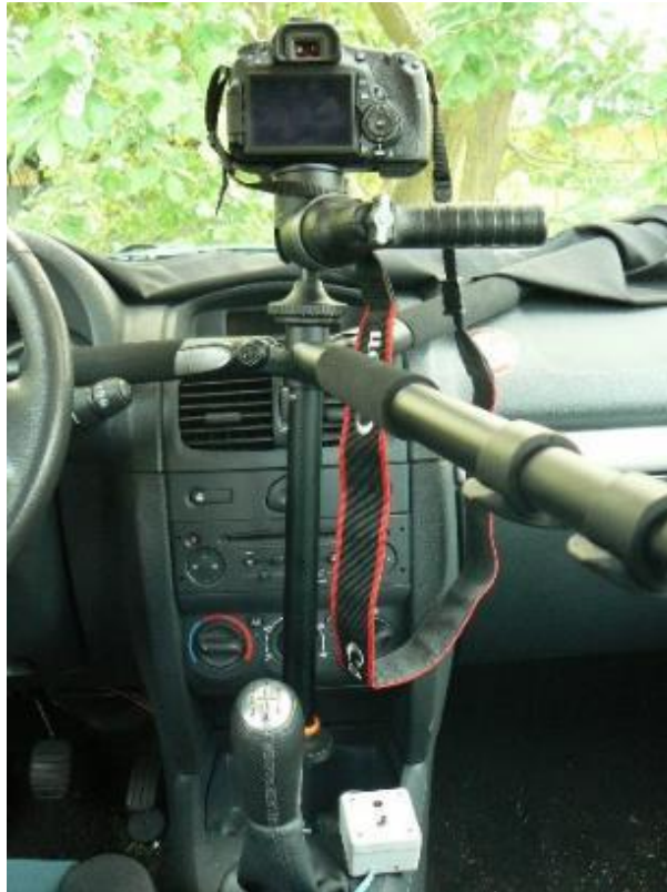
Figure 6.303 - View of the digital camera (canon EOS 60D) used to make videos from where the pictures have been extracted. A black protection has been placed on dashboard in order to minimize reflections.
