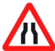
Figure 6.325 - P-17 vertical sign, narrowing on the road"
